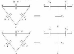
Where  $C_1 = 126 \ \mu\text{F}$ ,  $C_2 = 28 \ \mu\text{F}$ ,  $C_3 = 42 \ \mu\text{F}$ ,  $C_4 = 42 \ \mu\text{F}$ ,  $C_5 = 147 \ \mu\text{F}$ , and  $C_6 = 32 \ \mu\text{F}$ . Now the total equivalent capacitance is:
